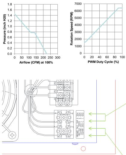
The external fan speed can be controlled using pulse width modulation at a recommended 5KHz to 25 kHz frequency applied at terminal position 4 (SPD CTRL, brown wire). The TC-720 temperature controller can be used to provide this PWM signal to reduce the audible noise at low cooling demands (use 5400Hz frequency setting). Electrical ground to terminal position 4 will reduce fan speed.
